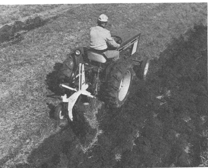
Small agricultural tractors have standard three-point hitches and are designed for continuous duty.
